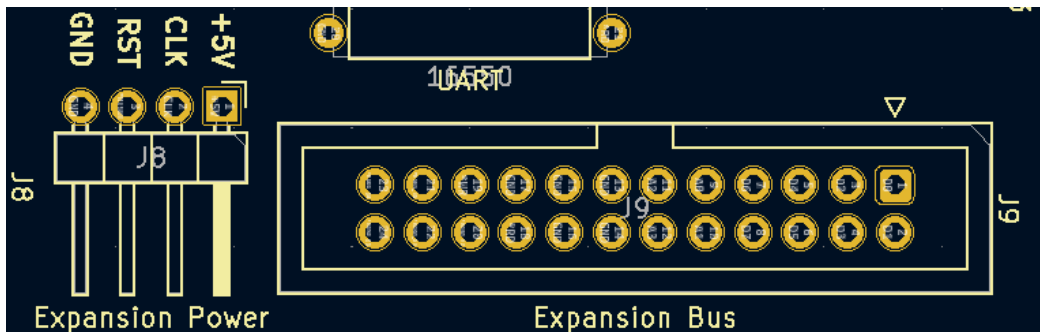
Figure 81 - Expansion Bus and Expansion Power
