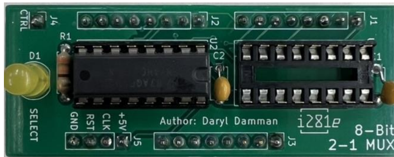
Figure 79 - Dip Package with and without Chips
